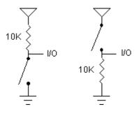
' Goto notpressed if button not pressed on Pin2 BUTTON PORTB.2,0,100,10,B2,0,notpressed
