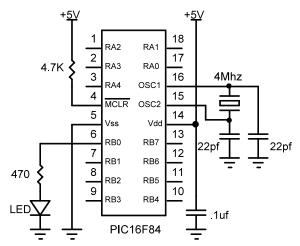
Build and double check this simple circuit on a protoboard and plug in the PIC MCU you just programmed. Our line of **PICPROTO**<sup>™</sup> prototyping boards is perfect for this kind of thing.
